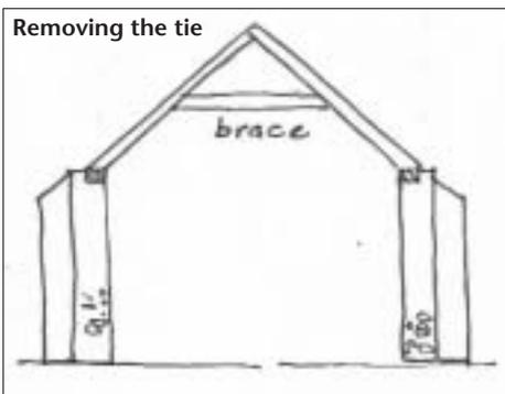
that appears to be in tension. When the wind blows, the brace in tension allows sufficient displacement to take place in the connection due to shrinkage, so as to prevent a tensile force developing. At the same time this transfers the load into the brace in compression and the dowels are not loaded in shear.
