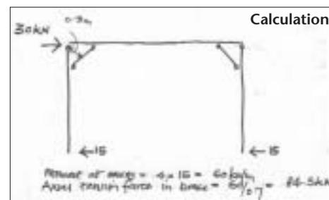
Making this as simple as possible we will assume a serviceability loading of 1kN/m<sup>2</sup> wind loading which will produce an eaves point load of 30kN. This assumes a horizontal loading on the roof.
