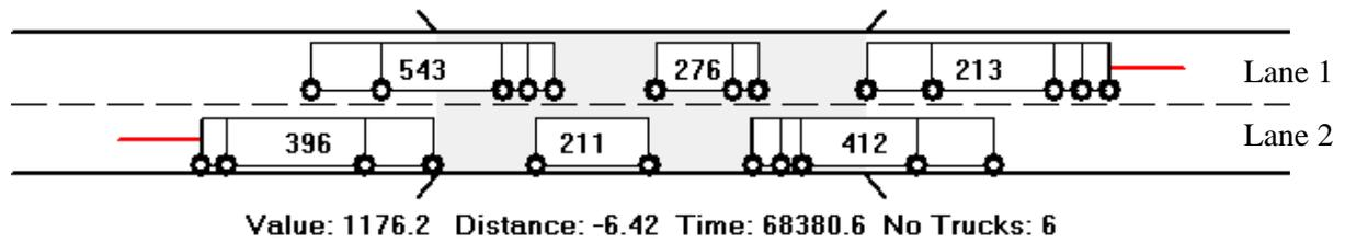
Figure 4: Sample maximum 2-hour congestion load event for the SCM-5 traffic model on 20 m bridge length, LE1 (mid-span bending moment on simply supported span) (the numbers on the trucks are the GVW in deci-tonnes).
