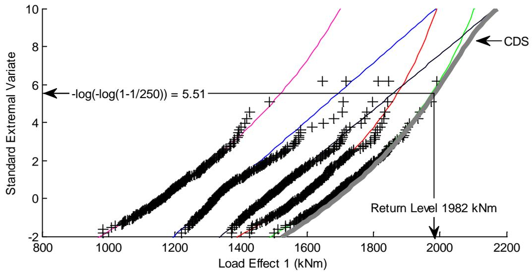
Figure 6: Example fit and extrapolation on Gumbel probability paper to expected annual maximum load effect showing different loading event distributions and the resulting composite distribution (CDS) for LE1, bridge length 20 m, SCM-5.
