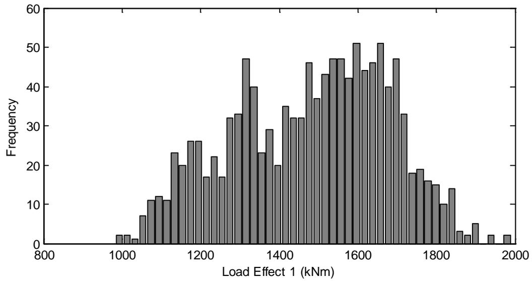
Figure 5: Histogram of 2-hourly maximum load effects, LE1, bridge length 20 m, SCM-5 traffic model.
