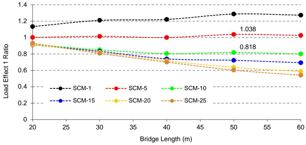
Figure 9: Ratio of SCM load effects to IDM-1 load effects for LE1, 0% cars.
