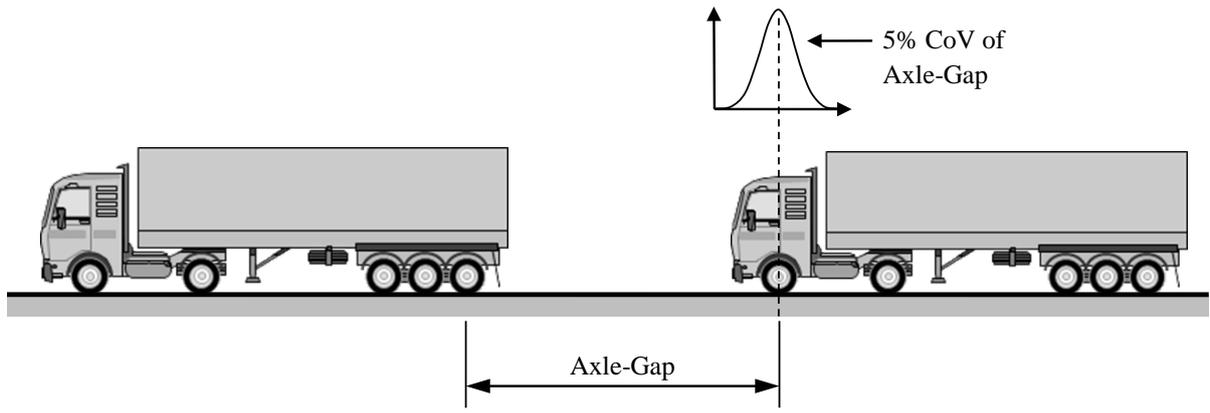
Figure 3: Simple gap model description showing nominal gap and variation.
