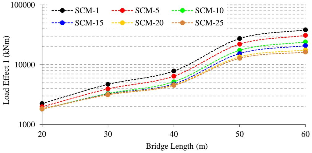
Figure 7: Load Effect 1 results for all SCMs and 0% cars.
