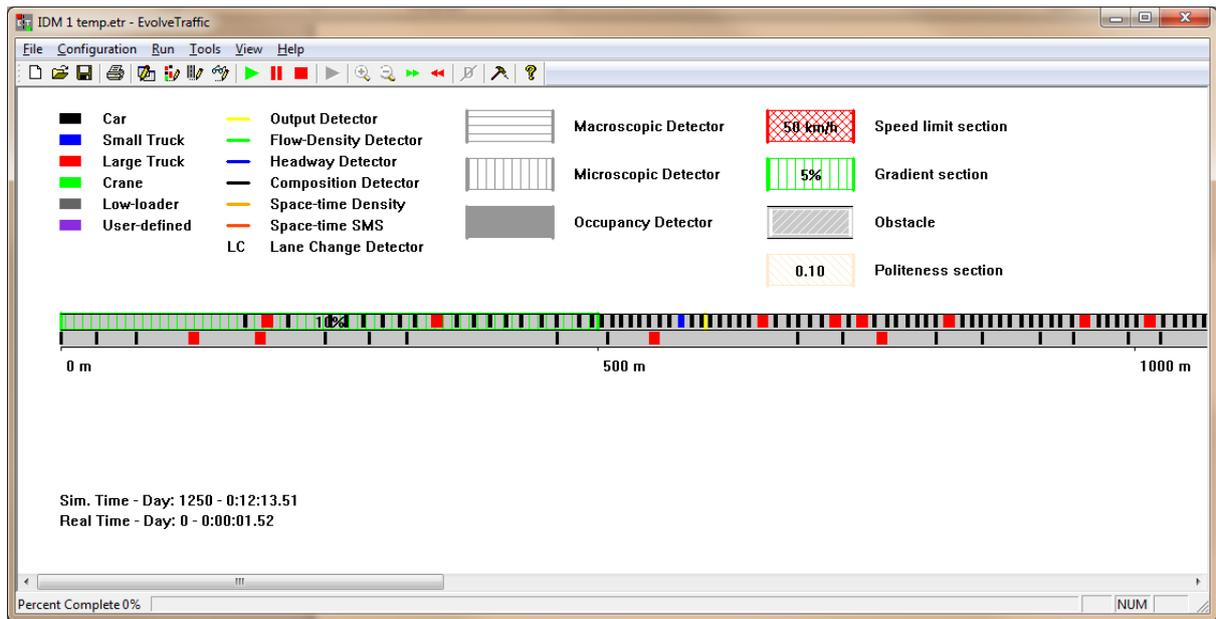
Figure 2: Screenshot of microsimulation illustrating formation of vehicle queue behind the inhomogeneity in the negative (top) direction (note the width of the vehicles is not to scale).
