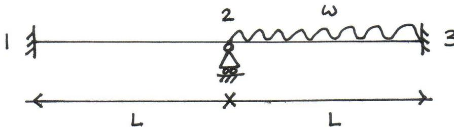
Firstly we construct the global matrix and restrict it. We know that there can be no vertical displacement, horizontal displacement or rotation at nodes 1 or 3. Also, there can be no vertical or horizontal displacement at node 2. Therefore, the only degree of freedom is the rotation at node 2.
