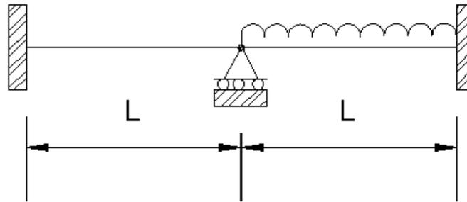
To analyse the beam it is assumed that there is a hinge at the pin support, a  $1\text{kNm}$  moment is then placed at either side of this.
