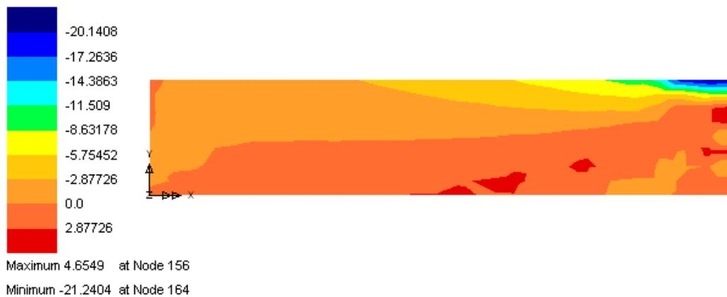
**Fig.2 Stress in beam at failure**
