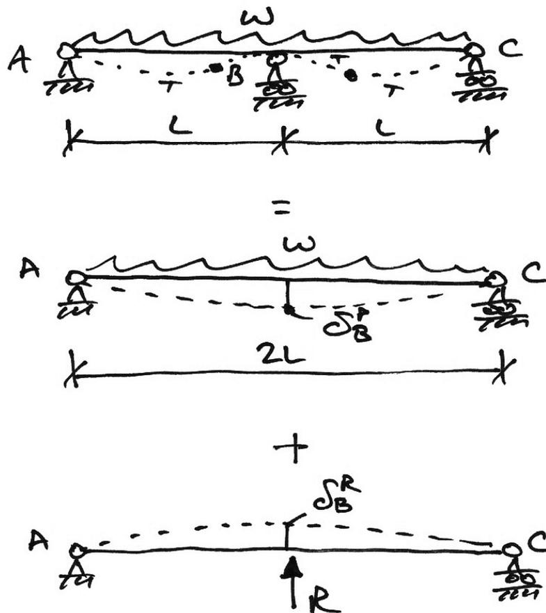
Once again we use compatibility of displacements for the original structure to write:
