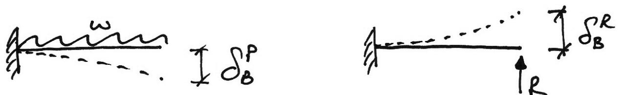
Now by compatibility of displacements for the original structure, we know that we need to have a final deflection of zero after adding the primary and reactant deflections at  $B$ :
