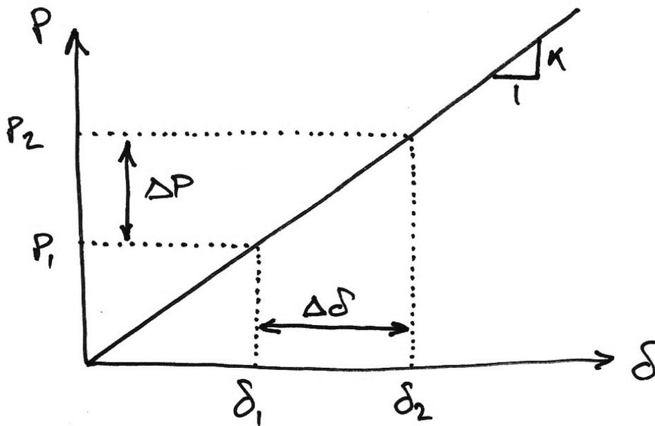
For an initial load on the structure we have:
